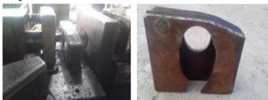
Fig.1 Die Block Failure
