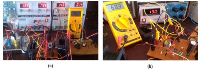
Fig.22. Complete Hardware Setup of TIESC-SC Converter (a). without snubber inductor (b). with snubber inductor
