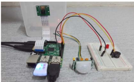
Fig.4. Motion detecting camera security system experimental setup
