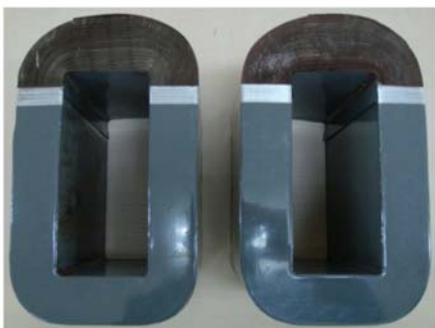
Fig 2.1.a. single phase transformer
