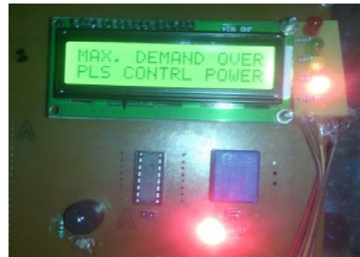
Fig 2. Photograph of maximum demand control on exceeding the desired maximum demand
