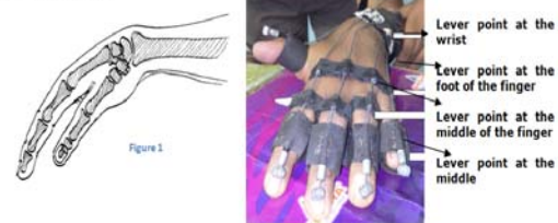
Stage1: Identification of the lever point of fingers in order to actuate as shown in figure
