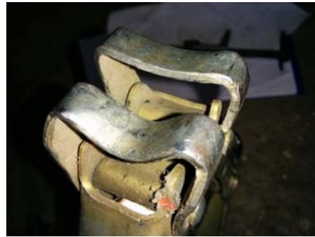
Fig. Failure of Jack Head
