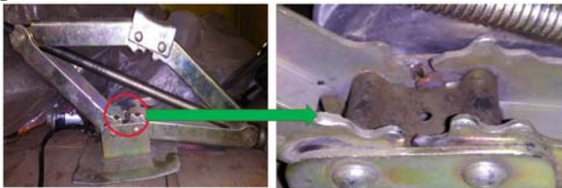
Fig. Failure of Screw and Arm Teeth
