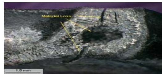
Fig. 5 Hollowing out of a polyacetal hinge due to acidcatalyzed Hydrolysis. [2]
