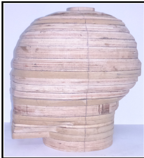
Fig. 11 Step6 - Headform takes shape after joining all Plates
