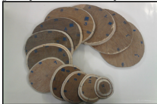
Fig. 9 Step4 - Edges grinded according to markings in Step3
