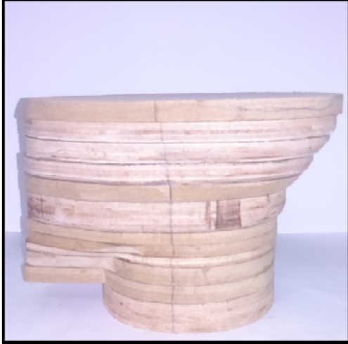
Fig. 10 Step6 – Joining done using glue and nails
