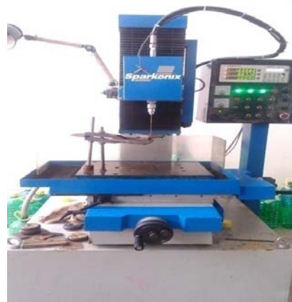
Fig.1: Photograph of special purpose EDM drill machine (EDD 44)
