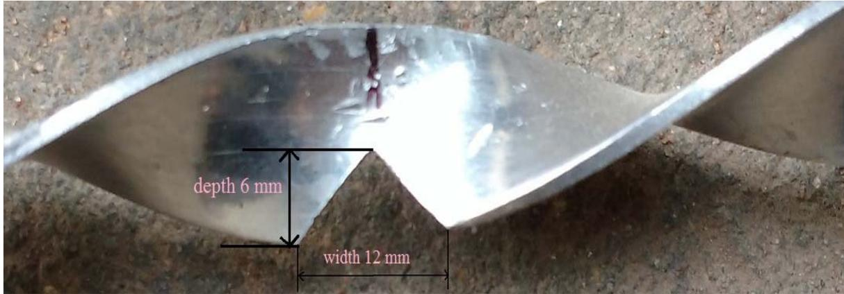
Fig.2. Photograph of v-cut twisted tape inserts
