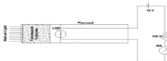
Fig.3.17: circuit setup for light transmittance test
