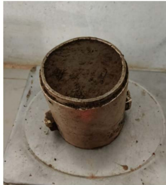
Fig 3.9: Mould after the filling of soil
