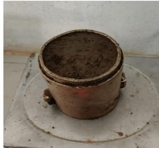
Fig. 4.6: Mould after the filling of soil
