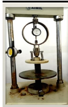
Fig. 4.8: Unconfined Compression test apparatus.
