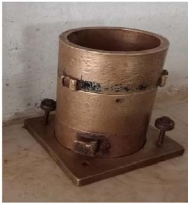
Fig. 4.5: Proctor compaction test apparatus
