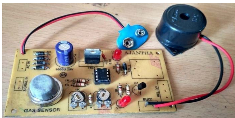
Figure 3: LPG leakage detection and alert system
