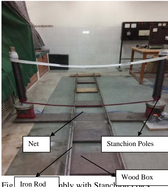
Fig. Iron Rod assembly with Stanchion Poles
