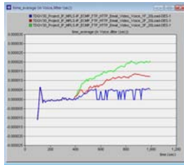
Figure 11: Voice Jitter: Increases because of link failure and increase in the network load.
