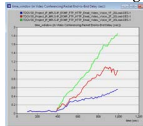
Figure 10: Video conferencing packet End to End Delay under mutation testing and network loading.
