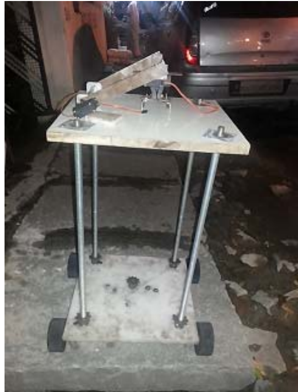
Fig.6: Nylon base with screw rods, wheels, platform and gripper
