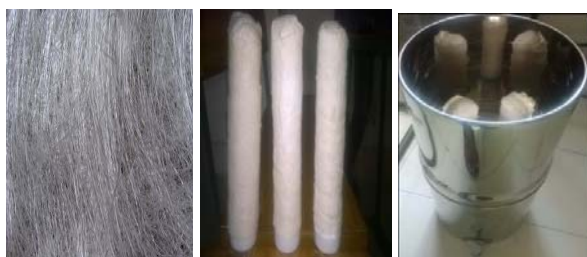
a) fibreglass mat b) after encircled filter candle with fibreglass mat c) filter candles fixed in water filter
