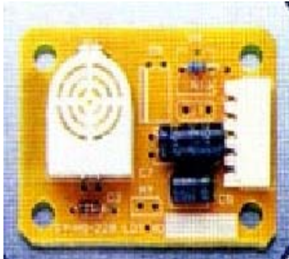
Figure (4): Humidity sensor
