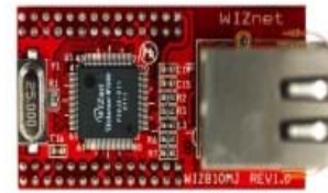
Figure (6): Ethernet Module
