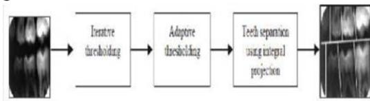
Figure 7 Block diagram of segmentation algorithm [17]
