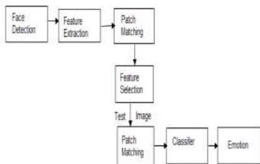
Fig 4.Steps for emotion detection using patches
