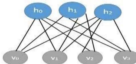
Fig9. An illustration of the layers and connections of an RBM
