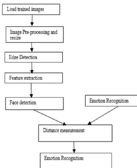
Fig 2. Functional block diagram of the facial recognition system.
