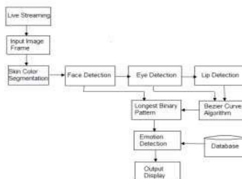
Fig 3. Steps for emotion recognition using Desktop Devices
