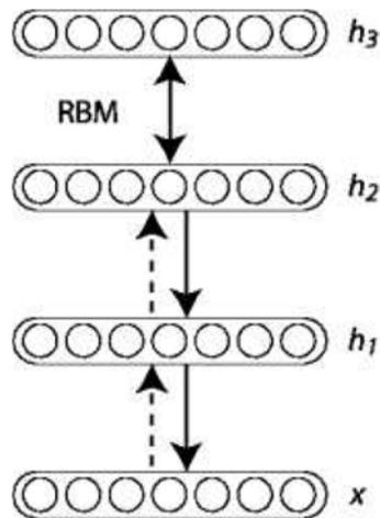
Fig10. A simple graphical illustration of a DBN with 3 hidden layers
