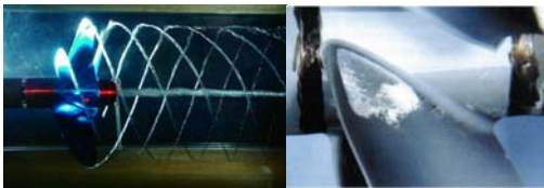
Fig.1 (a) Tip vortex cavitation (b) Blade surface cavitation
