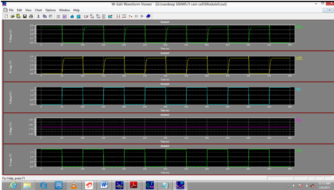
Fig8. Read/Write Waveforms of 64-bit SRAM Cell using 7T at 90nm
