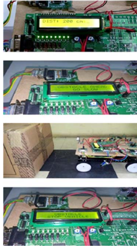
Fig. 5. Output of ultrasonic sensor is displayed on LCD
