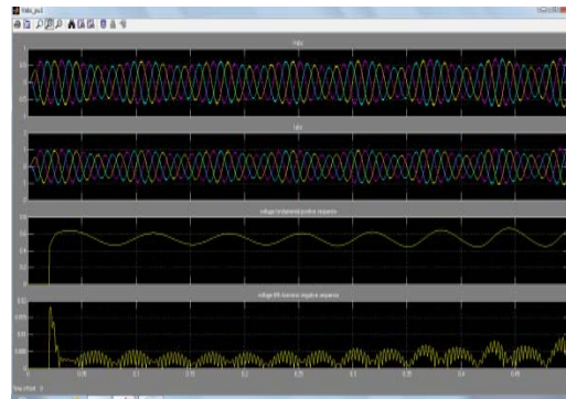
Fig 5: Three phase voltage, current, voltage fundamental positive sequence and 5 th negative sequence waveform using power quality analyzer 1(at load) of micro-hydro system supplying RL-Load
