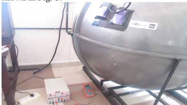
Fig. 5: Experimental setup for finding the effect of junction temperature on 6W LED string without heat sink
