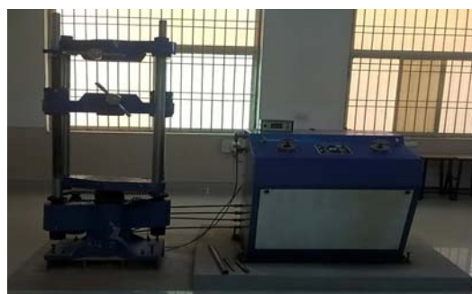
Figure 3: Experimental setup of fracture test
