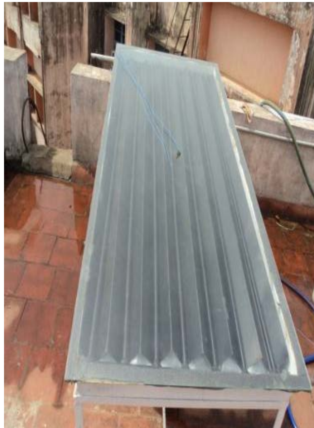
Figure 2. V-Grooved Absorber Plate Solar Water Heater
