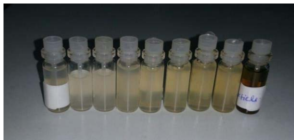
Figure 7: Change in the yellowness of the WW sample as volume of NPs added for treatment is increased from 0.5 ml to 6 ml per 50 ml of WW. Bottle 1 shows WW sample without addition of CoO NPs whereas, bottle 9 shows CoO NPs used for treatment.
