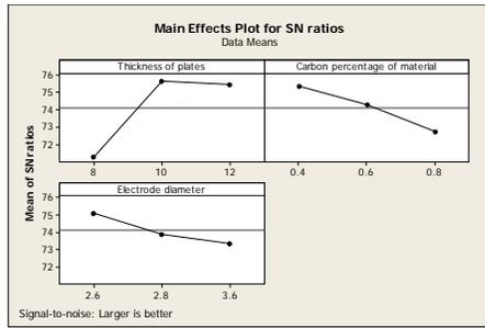
Fig-2: Graph between SN ratio, Thickness of material, Carbon % and Electrode Diameter
