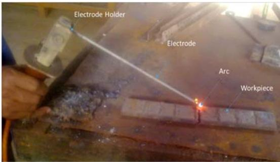
Fig.1.Electric Arc welding Process
