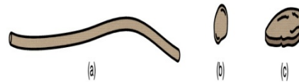
Fig 1.1 Possible physical shapes of imbedded phases in composite materials: (a) fibre, (b) particle, and (c) flake
