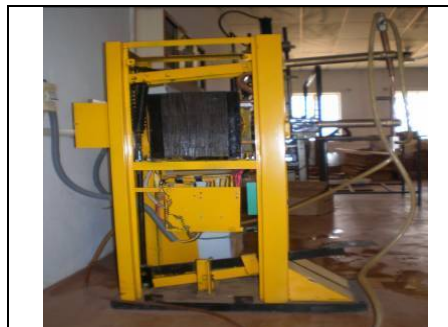
Fig. 5 KVA Spot welding fixture
