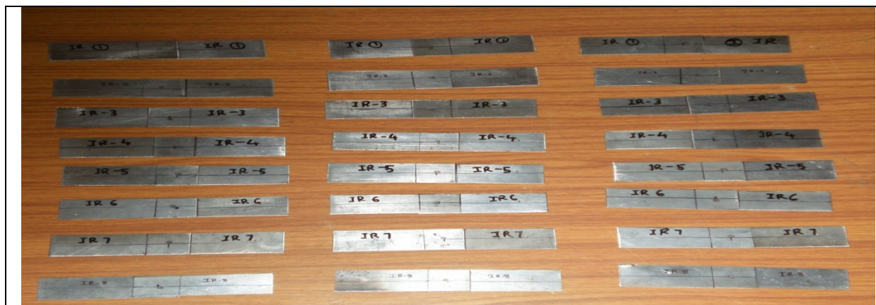
Fig. 6 Specimen samples of indirect resistance spot welding (IRSW)
