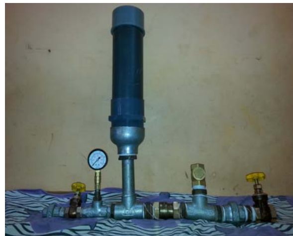
FIG 3.10 FINAL ASSEMBLE HYDRAULIC RAM
