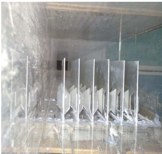
Fig.3 A channel with trapezoidal vortex generators
