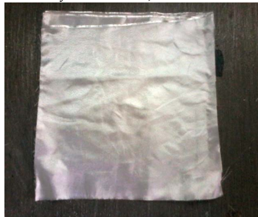
Fig. 1. Woven roving glass fiber sheet
