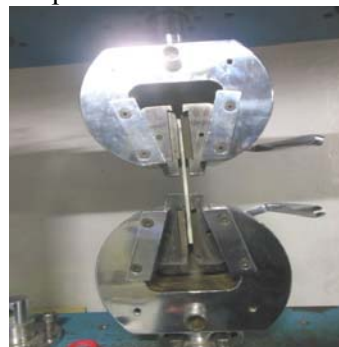
Fig. 4. Tensile test for finding material properties
