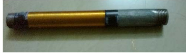
Figure 3. The search coil used for detecting the faults
