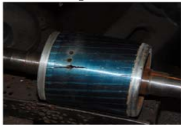
Figure 2. Artificially induced broken rotor bar fault
