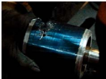
Figure 1. Drilling holes in the rotor
