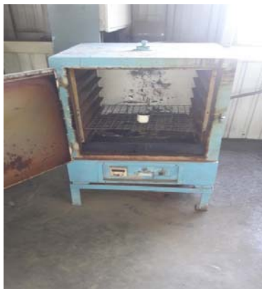
Fig.2.2: Assembly of Bio-oil taken in oven Weight of crucible=80gm Weight of oil with crucible=180gm
