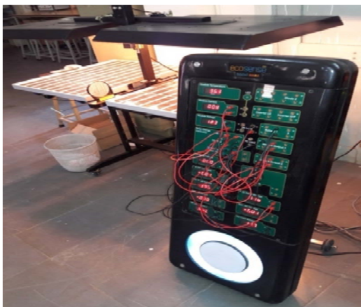
Fig.14(b) Controller connections for evaluation of I-V and P-V characteristics of series connected modules
