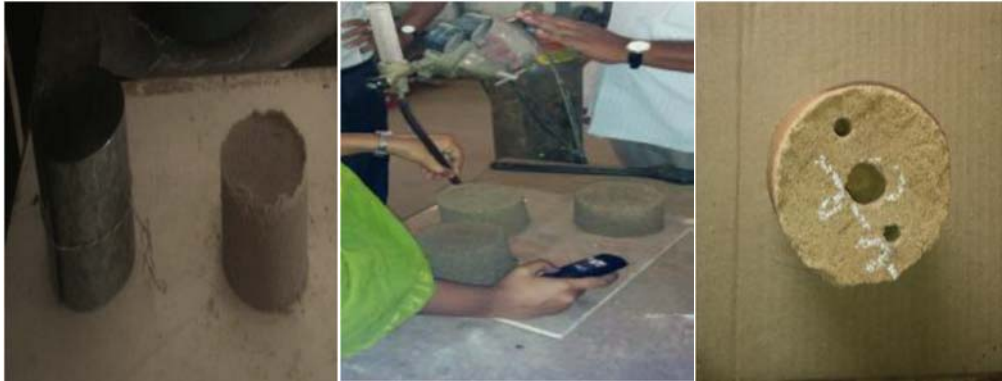
Figure 2 Mould Cavity of Sheet Metal with \text{CO}_2 silicate moulds Figure 3 Passing of \text{CO}_2 gas Figure 4 \text{CO}_2 – Silicate Mould after drilling process.
