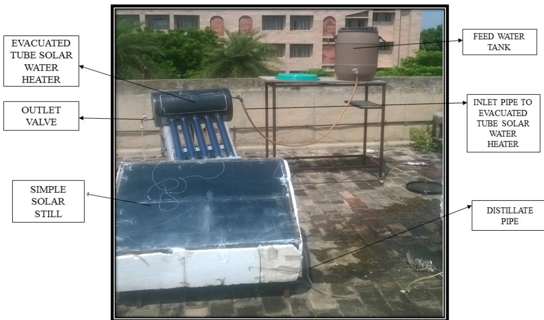
Fig.5. Direct flow through type evacuated tube solar collector coupled with simple solar still
