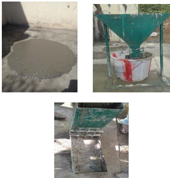
Fig-5.1: Fresh properties of Self Compacting Concrete
