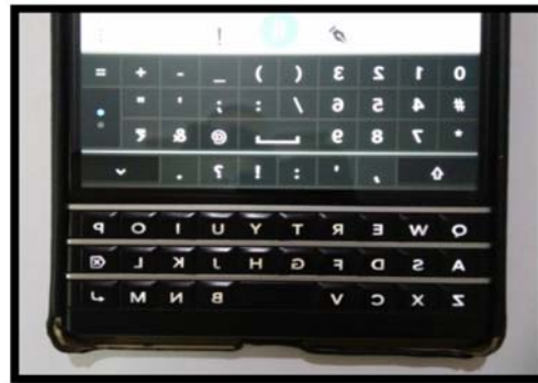
Fig. 4 Blackberry Passport Physical and Touch Screen (In extension to physical one) Keypads
