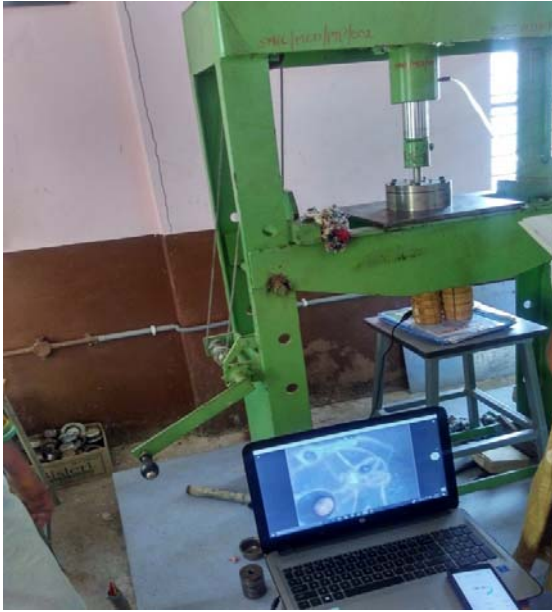
Fig.3 Setup used for formability test
