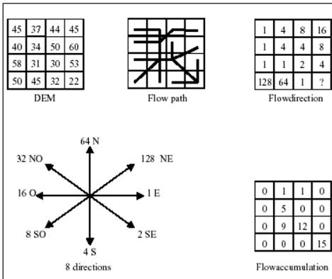
**Fig.6:** Flow Accumulation grid generated from flow direction grid
