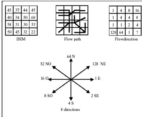
**Fig.5:** Mechanism involved in the generation of Flow direction grid from depressionless DEM
