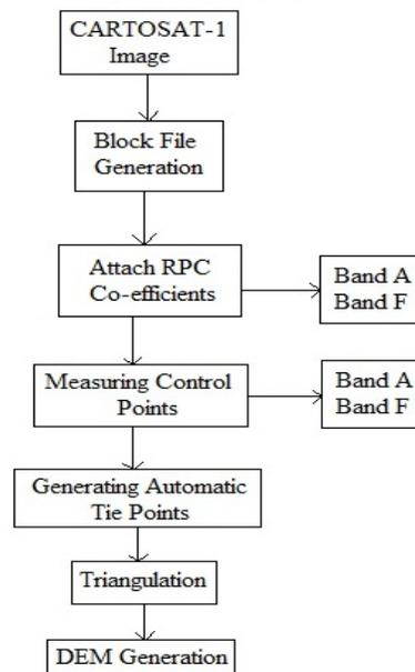
**Fig.3** : flow chart showing the automated extraction of DEM from Cartosat-1
