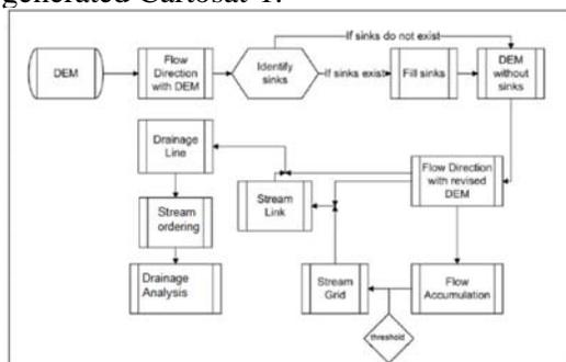
**Fig 4:** Flow chart for automatic drainage extraction
