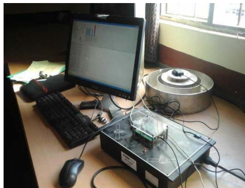
Fig 2: A typical experimental setup of GPS Receiver Kit, Software used, and Ring choke Base, Receiver Patch Antenna for investigation of SNR.
