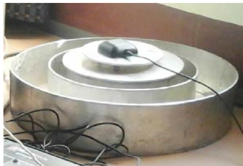
Fig. 3 Diagram Showing Ring Base Antenna prepared from Aluminum
