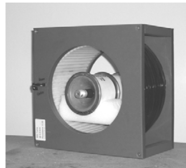
Fig. 7 A vacuum interrupter in position in the solenoid coil.
