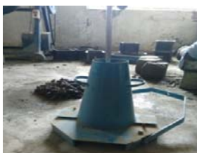
Fig 1 Slump Cone Test
