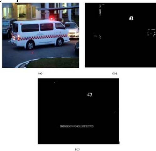
Fig:1.a) Image of a vehicle during daytime, (b) Detection of all lights, (c) Emergency vehicle detected
