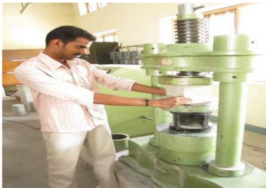
Fig 3 Specimen placed in CTM
